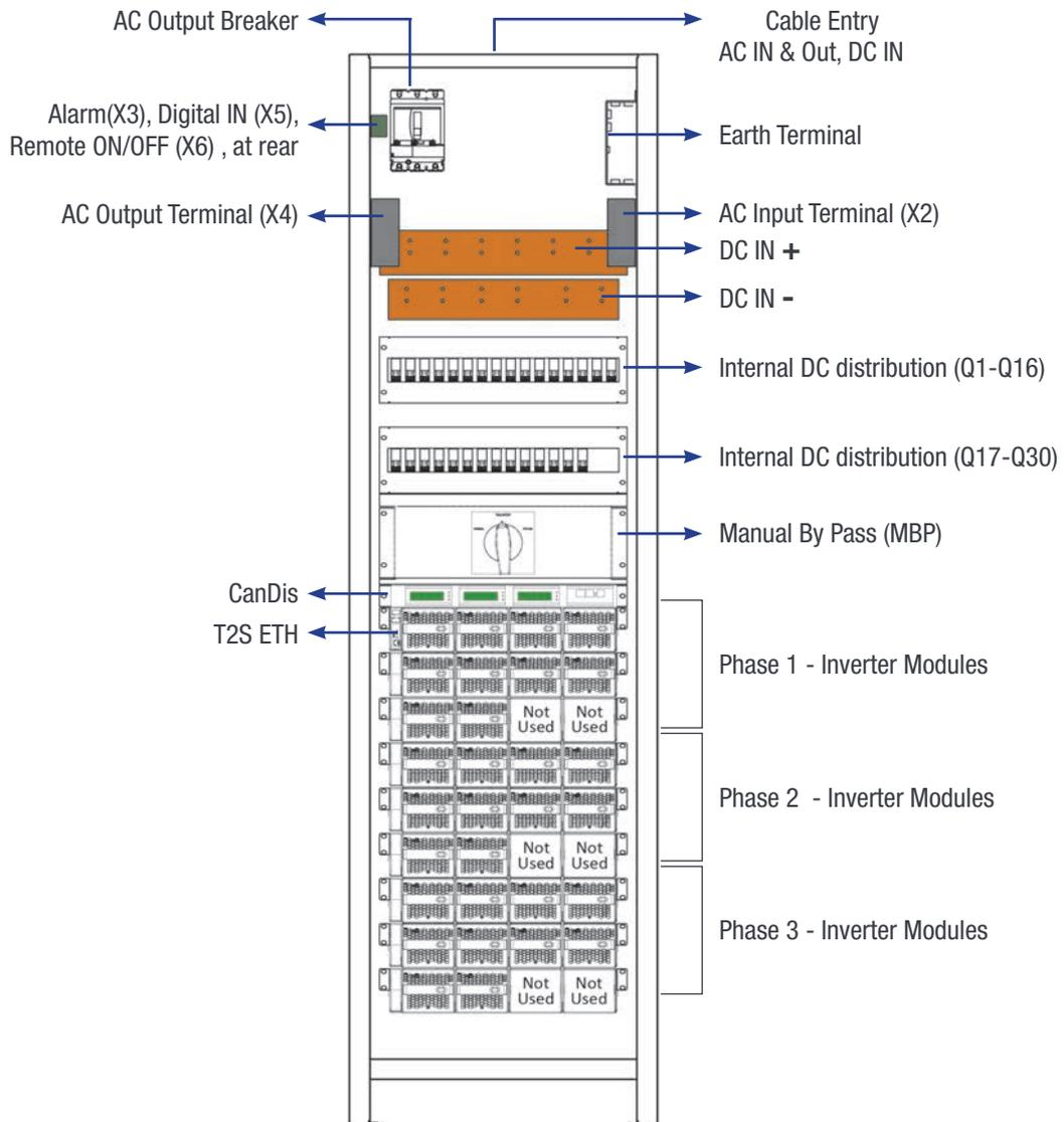
*Bravo EQZ4 90 kVA Inverter System - General Arrangement*
